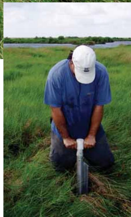
**Kyle Kelso** plunges a Russian peat corer into the ground at Sabine National Wildlife Refuge to recover a core sample. Core data are being used to determine whether specific wetland areas have eroded or subsided relative to sea level.
