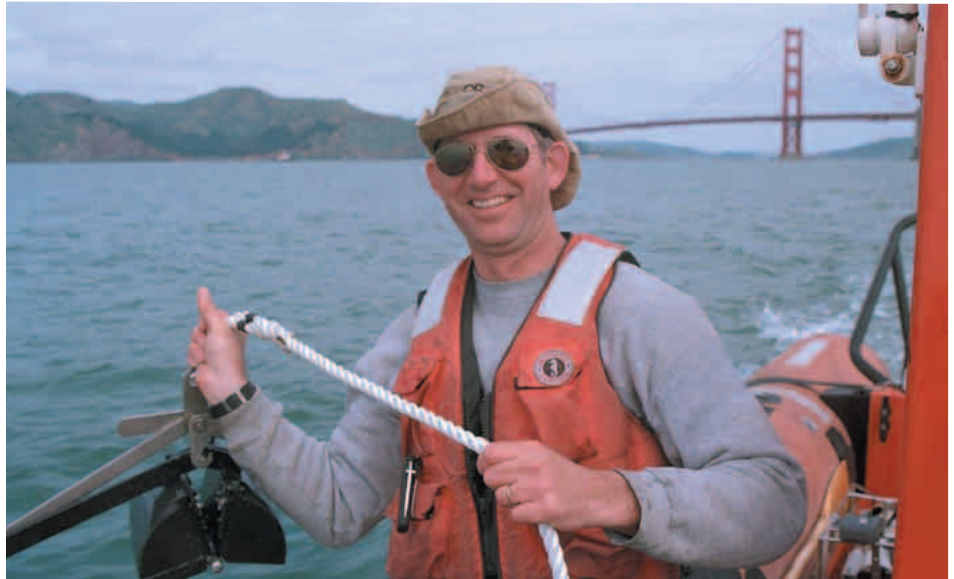
Dann Blackwood (Woods Hole) prepares a small van Veen grab to sample sediment from the Rigid-Hull Inflatable Boat aboard the NOAA ship McArthur near the Golden Gate Bridge. The nearshore sample will provide information about contaminants and sediment chemistry near the mouth of San Francisco Bay, thus rounding out the offshore sampling grid. Photograph by Gunnar Lauenstein (NOAA).
