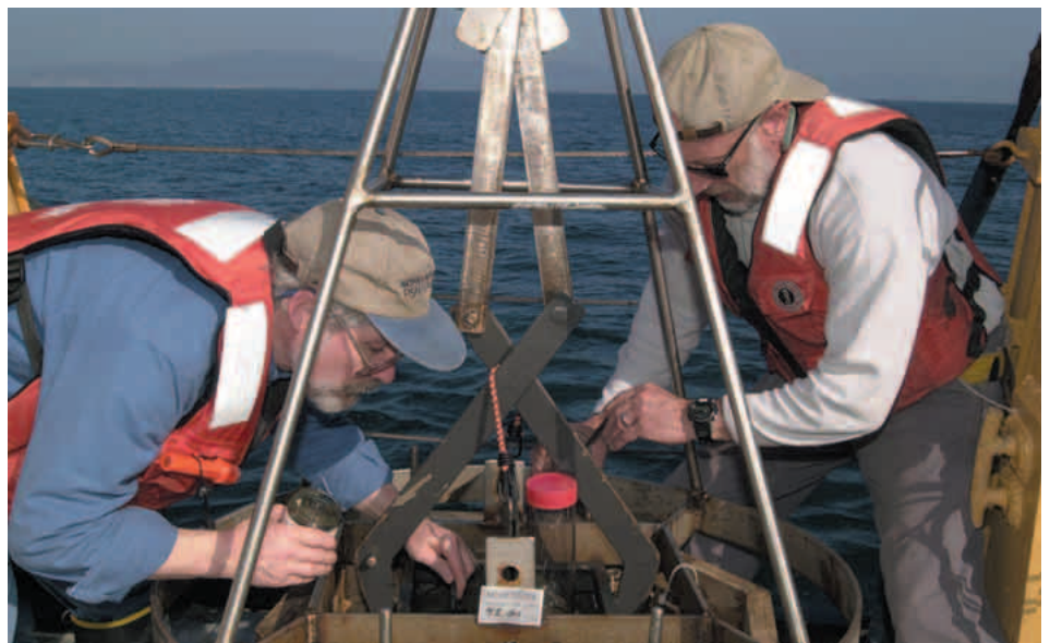
Ian Hartwell (left) and Mike Torresan subsample the upper surface of a sediment sample in a large van Veen grab. Photograph by Dann Blackwood .
