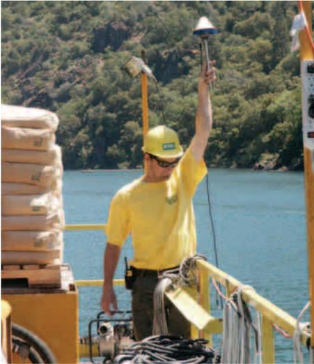
**Noah Snyder** holds a GPS (global positioning system) antenna to record the precise location of a core.
