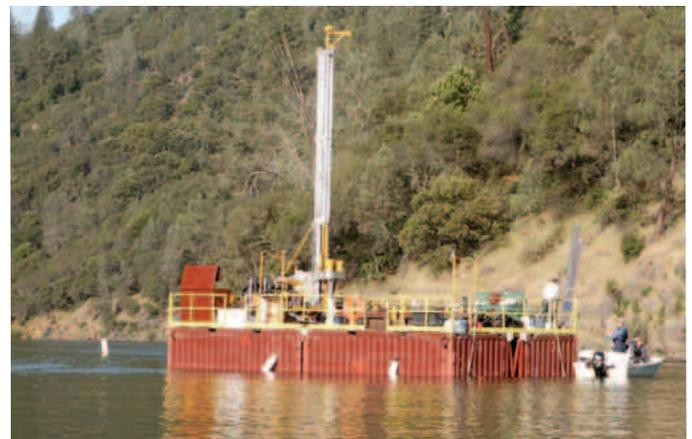
The DOSECC (Drilling, Observation and Sampling of the Earth's Continental Crust, Inc.) drill rig.
