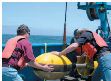
Ray Sliter (left) and Mike Boyle maneuver the 12-kHz fish back into its cradle after two weeks' steady duty.
