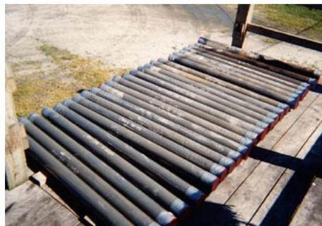
*Core sections recovered from the Rodanthe, NC, drillsite awaiting transport back to the North Carolina Geological Survey repository in Raleigh.*
