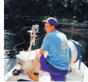
USGS hydrologist Jerry Casile (Reston, VA) collects spring-water samples for age-dating analysis.
