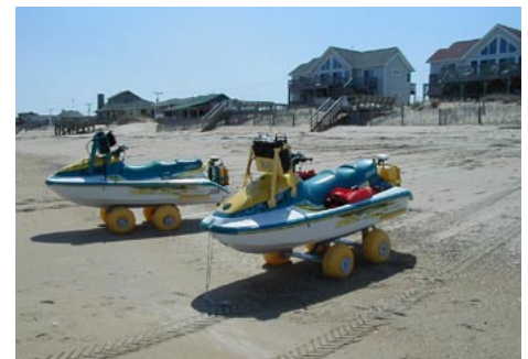
USGS bathymetric-surveying systems used by Peter Ruggiero and crew to measure cross-shore profiles during coastal-erosion research in North Carolina.
