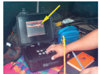
A control unit of the GSSI SIR-2000 system on the back of the truck records and stores digital images of the shallow subsurface structure of coastal sediment. The irregular orange reflector (arrow) is the contact between Holocene beach and dune sand and underlying Pleistocene beachrock. Photograph by Wayne Baldwin .
