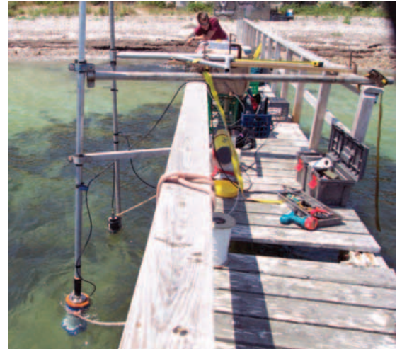
Testing the PCADP and ADCP off the dock to determine the best setup. Steve Ruane is in the background.
