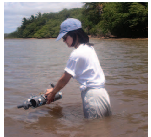
Connie Hoong uses a Niskin bottle to collect a water sample in muddy nearshore waters.
