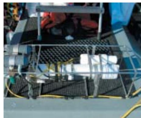
The towed instrument package includes camera, light, lasers, CTD (conductivity, temperature, depth) sensor, and optical-backscatter sensor.
