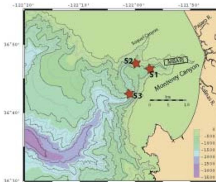
*Monterey Canyon, CA, showing the location of USGS subsurface moorings deployed from December 2002 to November 2003 (S1, S2, and S3) and the area where MBARI deployed instrumented frames on the canyon floor during the same period (box labeled "MBARI").*
