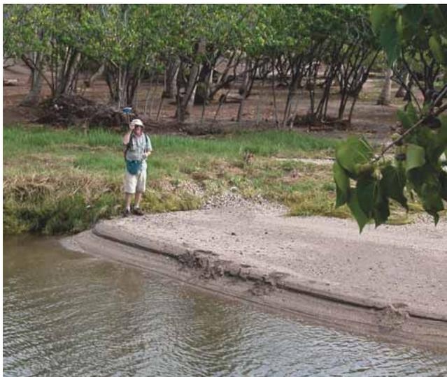
**Bruce Richmond** mapping an ephemeral flood-delta deposit at Pu'ukohola Heiau NHS. His equipment includes a GPS receiver and antenna in a backpack, used to accurately map the spatial distribution of coastal landforms in the field.
