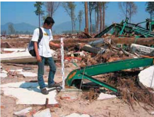
*Steel beam bent by debris carried in the powerful waves that struck Lho Nga on Sumatra's west coast. Photograph by Guy Gelfenbaum, USGS.*
