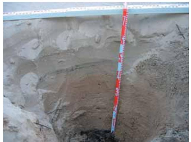
*Cross-sectional view of tsunami deposits at the village of Lam-puuk. A 73-cm thickness of sand was deposited over soil (dark material in bottom center), in beds indicating multiple pulses of sand deposition. The lowermost bed, 45 cm of sand grading upward from coarse to fine, settled from suspension in a single wave and can be used to characterize the wave's height and velocity. Photograph by **Guy Gelfenbaum**, USGS.*
