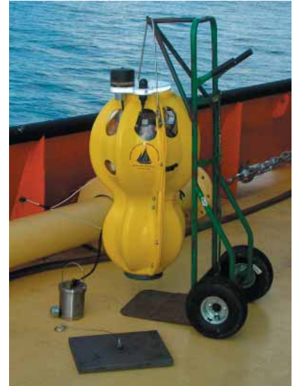
USGS-WHOI ocean-bottom seismometer, one of 10 instruments deployed in the Puerto Rico Trench.
