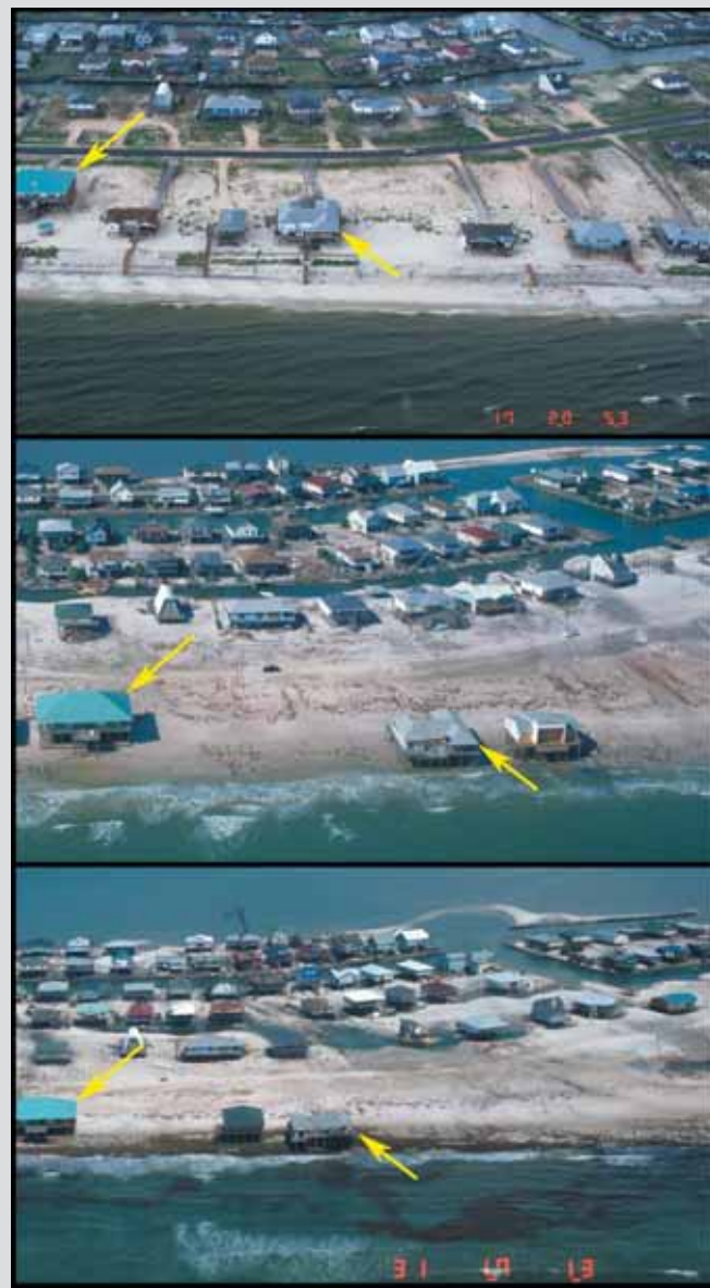
Dauphin Island. ► The top image was taken in July 2001, before Hurricane Lili (2002). The middle photograph was taken on September 17, 2004, immediately after the passage of Hurricane Ivan. The bottom image was acquired on August 31, 2005, two days after Hurricane Katrina. Note the road and two parallel canals in the first photograph. The post-Ivan photo shows overwash deposits covering the road and encroaching on the first canal. The post-Katrina photo shows that the overwash deposit has not only covered the road but also filled the first canal and is encroaching on the second. The beach appears brown in the bottom photograph because of a "deposit" of plant debris.
