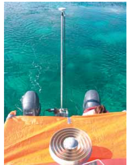
ATRIS survey underway. Ashtech Z-Surveyor antenna (bottom of photo) receives geographic signals for accurate positioning of the precision bathymetric system. The CSI MiniMAX antenna (top of photo) sits atop the along-track vessel-mounted sensor package. The sensor package mounted to the base of the pole under the sea surface collects photographs, video footage, depth data, and headings.
