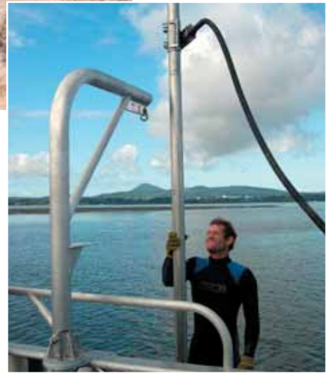
Eric Grossman operates a vibrocorer in northern Puget Sound as a flood tide races in.
