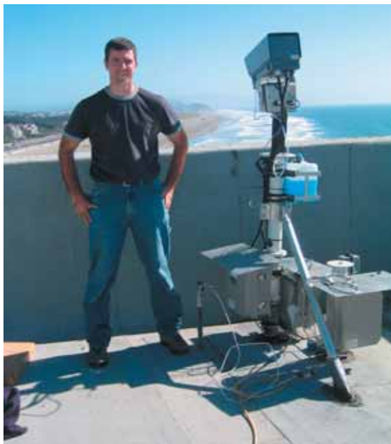
Patrick Barnard stands beside a Webcam that he and WCMG oceanographer Dan Hanes installed on the roof of the Cliff House Restaurant overlooking San Francisco's Ocean Beach. The camera records images of the beach, which Patrick and Dan use in their research (see URL http://walrus.wr.usgs.gov/coastal_processes/ ).
