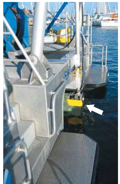
Interferometric sonar (arrow) mounted to the stern of the research vessel Shearwater.
