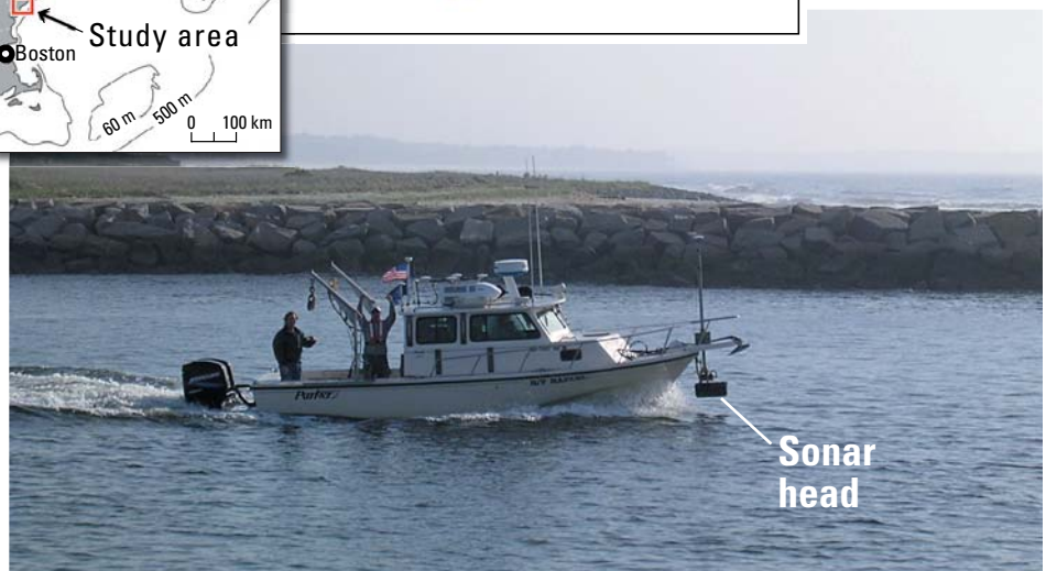
▼ The research vessel Rafael departs Wells harbor early on a foggy Maine morning. Rough seas caused flexing of the bow-mounted sonar head, which was reconfigured the next day and deployed farther aft on a side boom. During surveys, the sonar head is lowered into the water, where it rides about 3 ft under the surface. Photograph by Erika Hammar-Klose .
