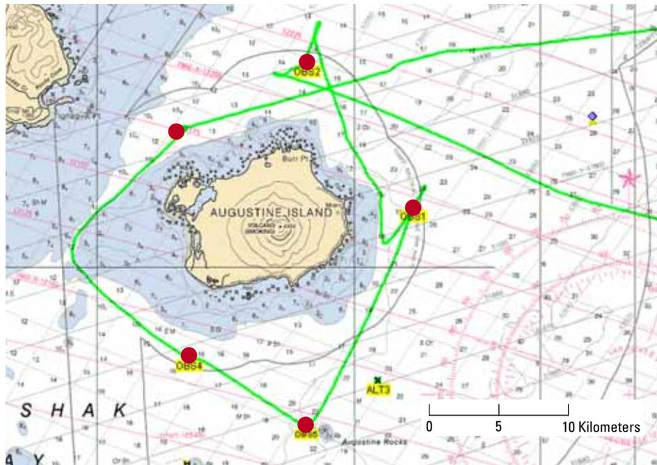
Approximate locations of ocean-bottom seismometers (OBSes) deployed on February 8, 2006. Red dots, OBS locations; green line, ship's path. Scale is approximate. Modified from image provided by U.S. Coast Guard cutter Roanoke Island.
