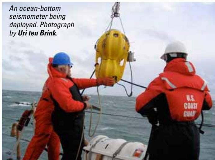
An ocean-bottom seismometer being deployed. Photograph by Uri ten Brink.
