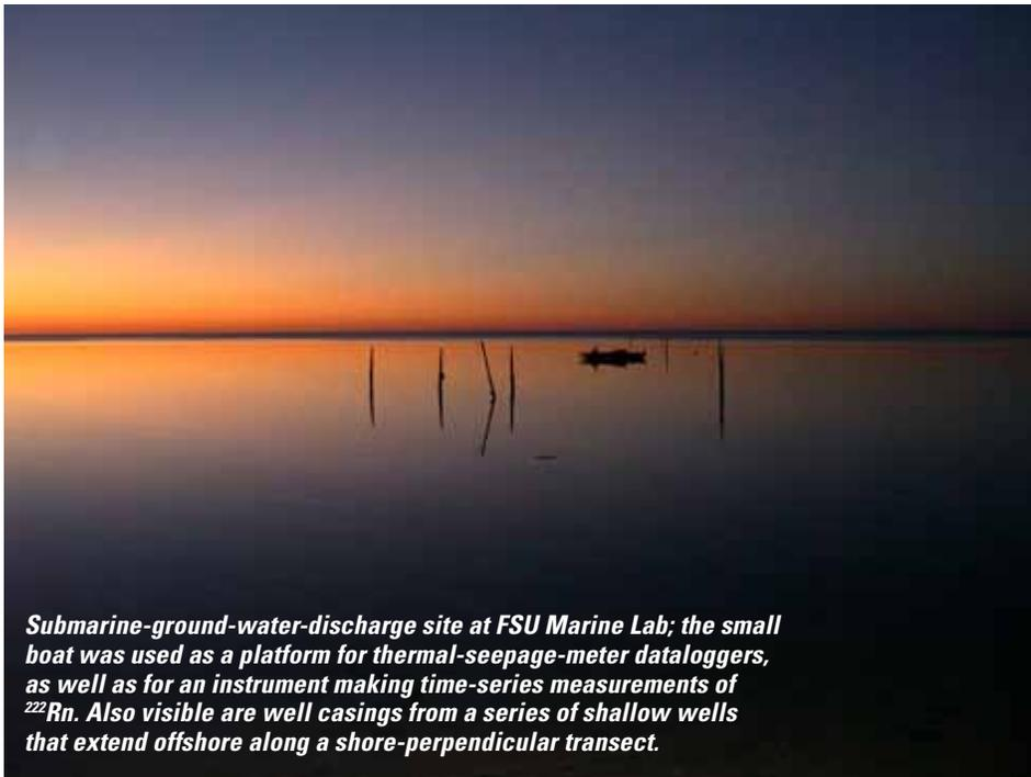
*Submarine-ground-water-discharge site at FSU Marine Lab; the small boat was used as a platform for thermal-seepage-meter dataloggers, as well as for an instrument making time-series measurements of <sup>222</sup>Rn. Also visible are well casings from a series of shallow wells that extend offshore along a shore-perpendicular transect.*
