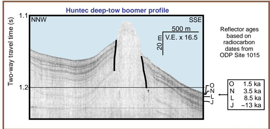
*Closeup of the mud volcano in a high-resolution seismic-reflection profile created from Huntec deep-tow boomer data collected by the Geological Survey of Canada in 1992. The boomer source and receiver were towed about 200 m below the sea surface; resolution is about 40 cm. V.E., vertical exaggeration.*
