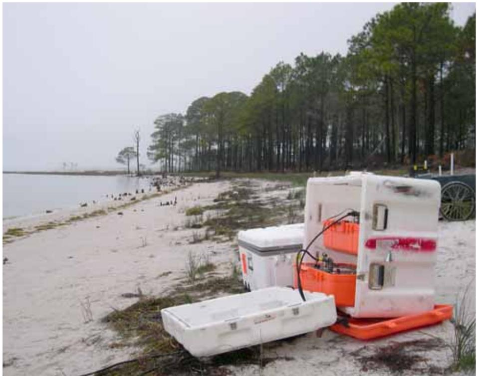
*Two electromagnetic-seepage-meter control panels on the beach close to the FSU Marine Lab.*
