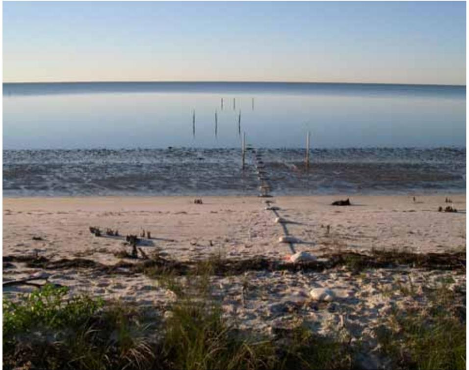
*Time-series resistivity cable, showing electrode spacing (one sand bag per electrode) across the freshwater/saltwater interface.*
