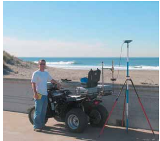
Jeff Hansen with an all-terrain vehicle (ATV) equipped with a geographic positioning system (GPS) used to measure topographic profiles of the foreshore. ❁
