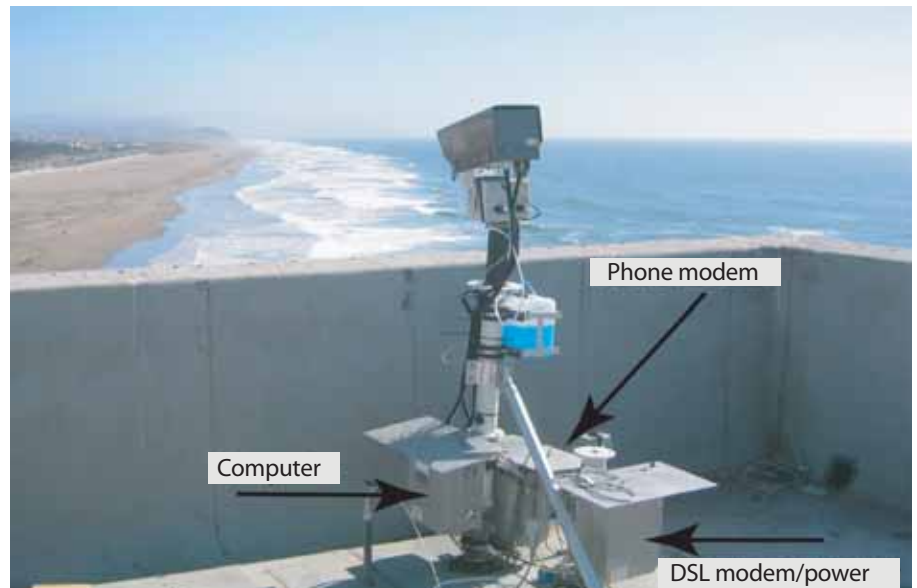
Video camera mounted on top of the Cliff House restaurant at the north end of Ocean Beach. DSL, digital subscriber line. Photograph by Ann Gibbs .
