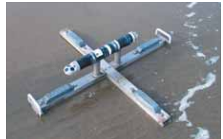
Nortek Aquadopp current profiler mounted on an aluminum frame (constructed by Kevin O'Toole at the USGS Marine Facility in Redwood City, Calif.). Two handles facilitate moving the apparatus. Sand anchors on the handle ends and tapered "feet" protruding from the frame bottom and embedded in the sand help keep the frame and instrument steady in the waves. Photograph by Patrick Barnard .
