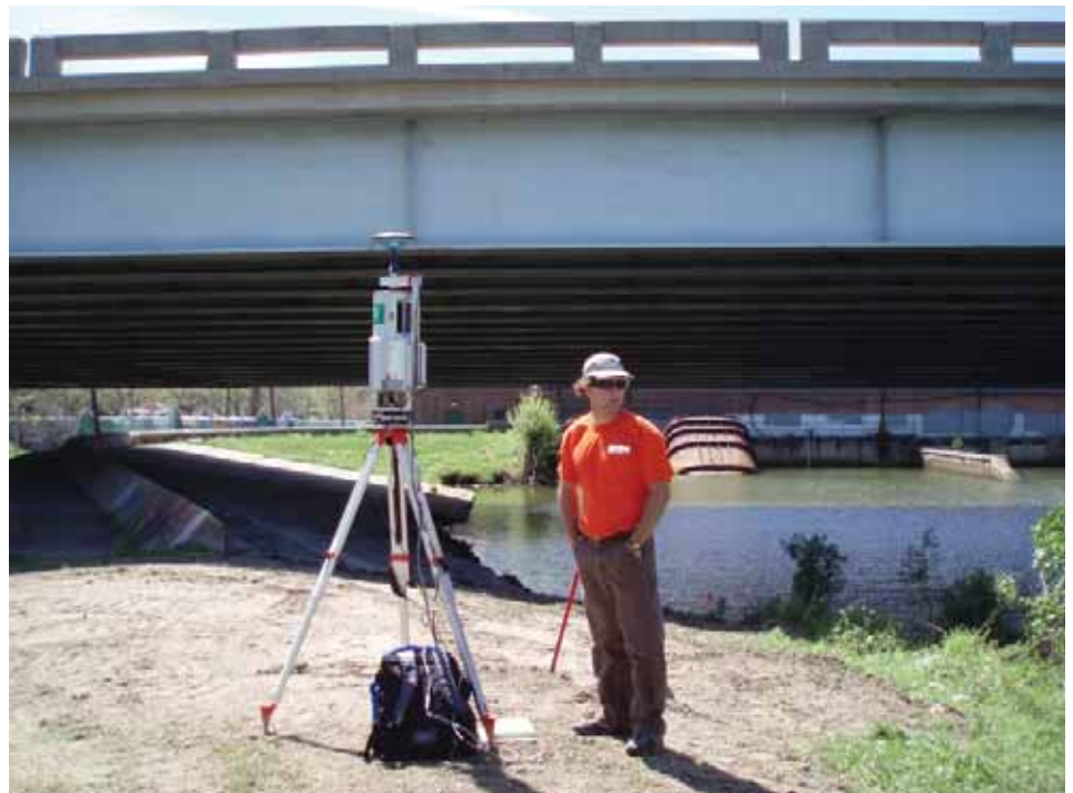
Brian Collins oversees simultaneous laser-scanning and differential global-positioning-system (GPS) surveys at the Orleans Avenue Canal pump station, a site that he and Rob Kayen did not include when they scanned levee breaks last October. The tripod supports both the laser-scanning unit (cylindrical instrument) and the GPS antenna (above the scanner). Floodwaters entered neighborhoods by way of the spillway beneath the highway overpass. The spillway had been designed to be several feet lower than the maximum floodwall elevation in the area in order to protect the pump station.
