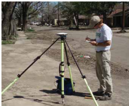
Brian Collins next to a GPS base station set up over a temporary control point near the 17th Street Canal levee breach. "Registration points" used to assign geographic coordinates to high-resolution laser scans were referenced off these temporary control points, which in turn were referenced off updated permanent benchmarks composing the geodetic control network in New Orleans.
