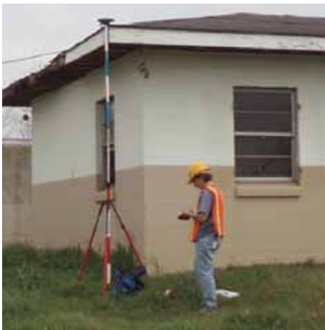
Diane Minasian collects GPS data from a roof corner, visible in the three-dimensional laser-scan data sets, near the Inner Harbor Navigation Canal (Industrial Canal) levee breach. Two breaches of the IHNC floodwall led to the flooding of the Lower 9th Ward district.
