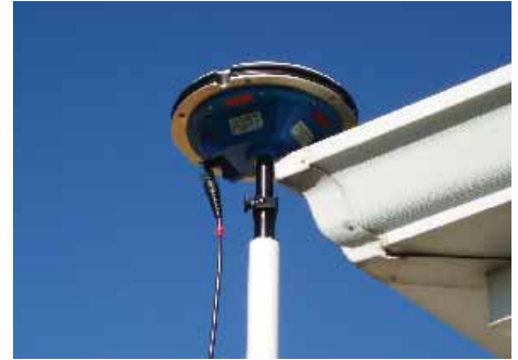
Close-up of the GPS antenna resting on one of the registration points (corner of a roof) near the 17th Street Canal levee breach.
