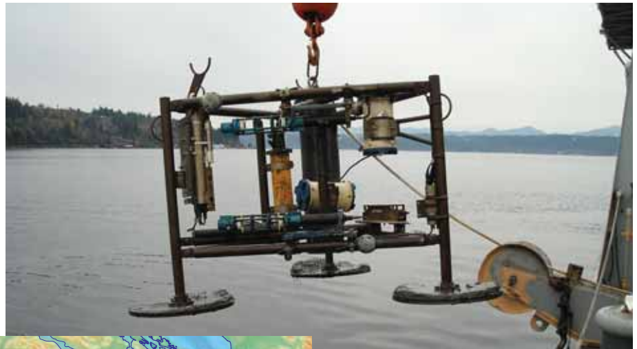
One of two instrumented tripods that sat on the floor of Hood Canal for 8 weeks in 2004, measuring such variables as current speed and direction in the canal's upper and lower layers, and near-bottom temperature, salinity, and water clarity. The second tripod (not shown) also held an instrument to measure near-bottom dissolved oxygen.
