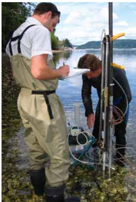
Seth Book (left) and Bill Simonds measure vertical hydraulic gradients along the shoreline of Hood Canal.
