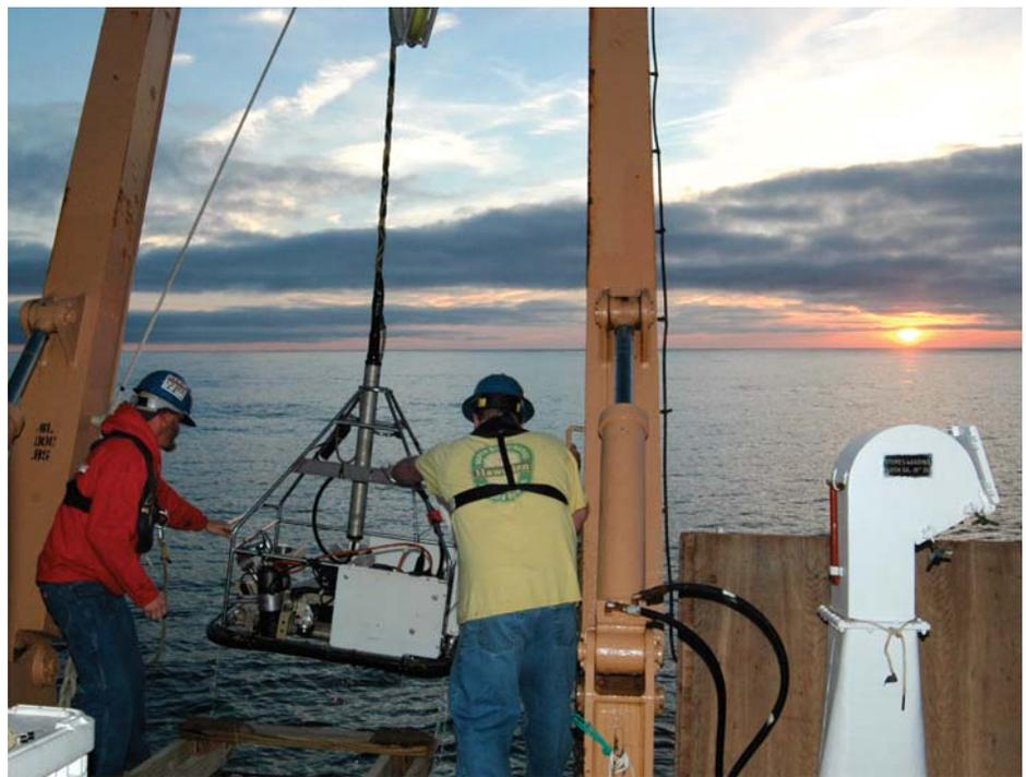
Crew members of the NOAA ship Delaware II in August 2006 deploying the USGS SEABOSS, a system for imaging and sampling the seabed that has video and still cameras and a grab for collecting sediment and benthic fauna. Photograph by **Dann Blackwood**, USGS.
