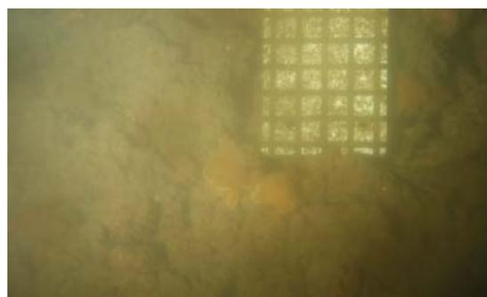
Image taken early in the study (top) shows no accumulated sediment on the block or turbidity in the water. Second image taken 1 week later (bottom) shows turbid water and an accumulation of sediment on the block.
