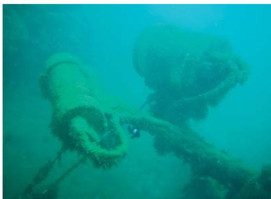
Photograph taken just before the instrument was picked up off the sea floor shows the system's components covered by algae and other organisms.
