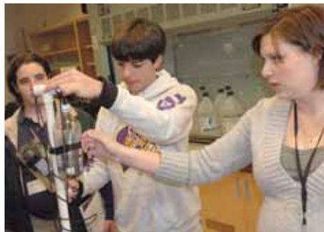
Job-shadow students **Quintin Brown** (left) and **Brock Minvielle** help biologist **Samantha Hill** assemble the microphone for a remote-recording device known as a “frog logger.” The microphone, protected by a plastic 2-liter soda bottle and connected to a personal digital assistant (PDA), allows researchers to remotely record the calls of frogs in their natural habitats and later analyze the recordings to determine species types and population densities.
