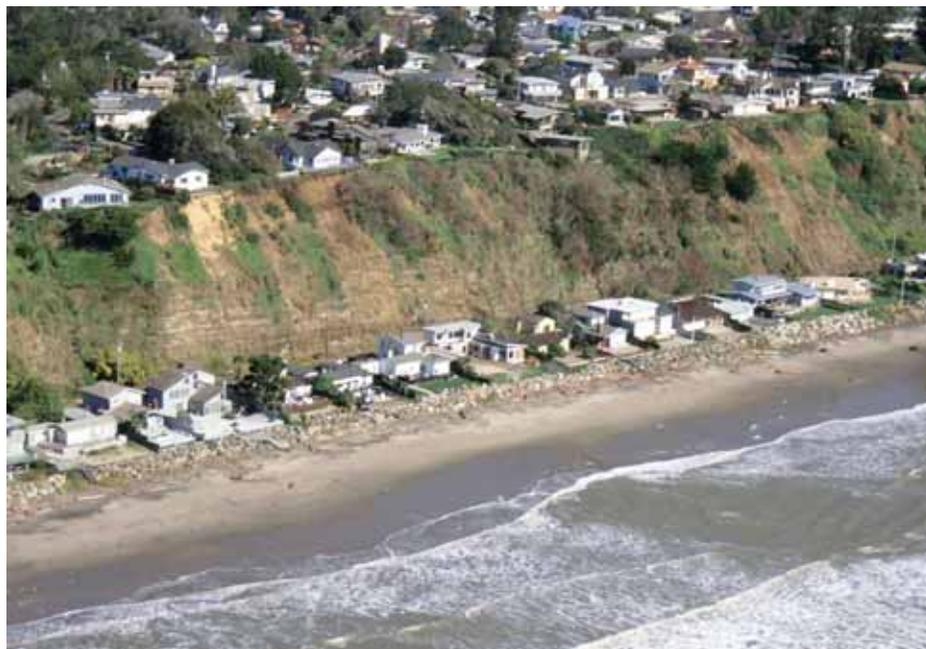
Oblique aerial view of a coastal cliff in Aptos, California, northern Monterey Bay, from the recent USGS report on coastal cliff retreat. Photograph taken by **Cheryl Hapke** in February 1998, after a major storm had triggered debris slides that damaged several houses at the base of the cliff.
