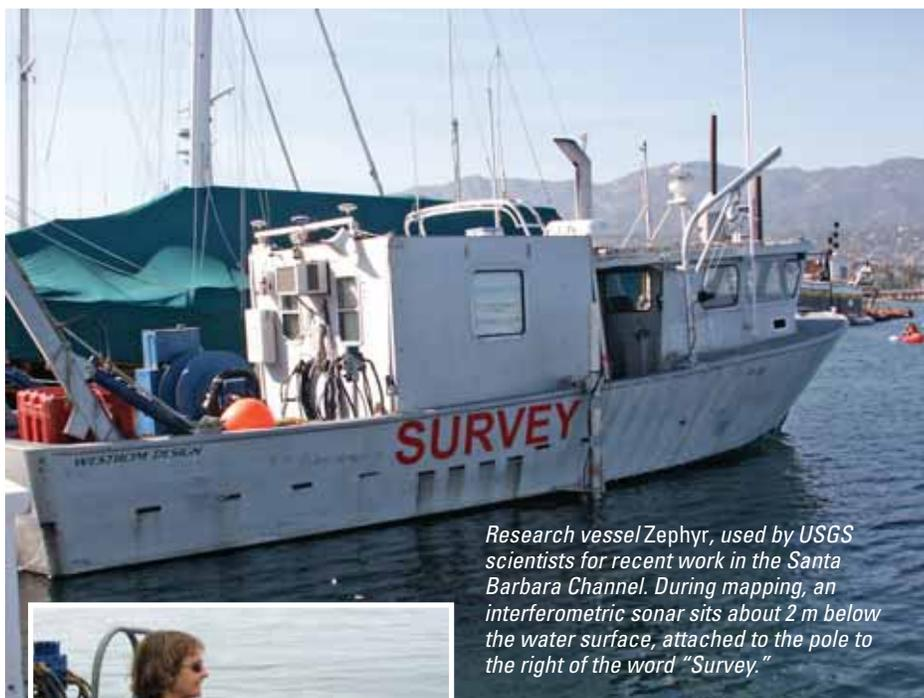
*Research vessel Zephyr, used by USGS scientists for recent work in the Santa Barbara Channel. During mapping, an interferometric sonar sits about 2 m below the water surface, attached to the pole to the right of the word "Survey."*
