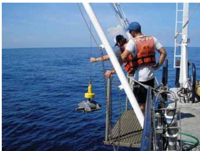
**Kevin Bradley** (left) and **Shane Dunn** of USF lower Shipek sediment sampler from the research vessel *Bellows*.
