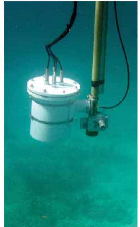
*◀ Hydrographic survey pole, which supports an acoustic transducer at its lower end and a GPS antenna at its top to collect data for bathymetric mapping.*
