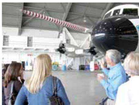
NOAA's P-3 research aircraft with "barber-pole" probe protruding from its forward end. In the early days of aircraft research, the probe was used to sample the air in front of the bow wake of the aircraft. More recent instrumentation has shown that it is more practical to sample the air immediately adjacent to the aircraft. The "barber pole" has remained on the aircraft and serves mainly as a lightning rod.
