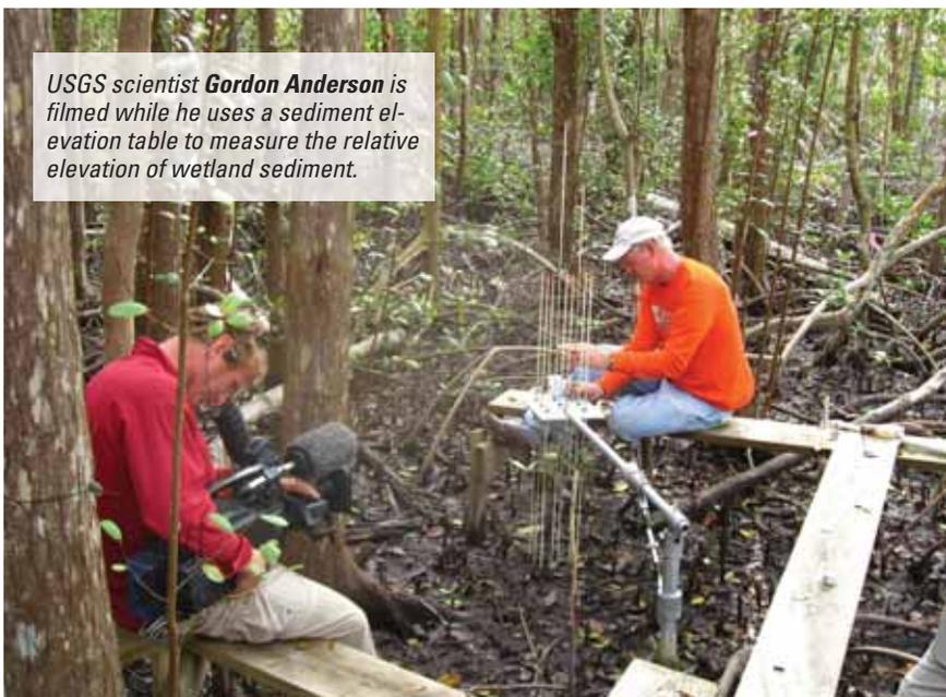
*USGS scientist **Gordon Anderson** is filmed while he uses a sediment elevation table to measure the relative elevation of wetland sediment.*
