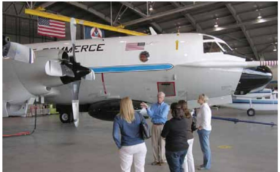
**Jack Parrish**, NOAA Aircraft Operations scientist, describes the capabilities of the P-3 to visiting USGS scientists. The engine props vary in pitch to change the speed of the aircraft. The black pod on the bottom of the fuselage is downward-looking weather radar that is lowered away from the main aircraft body in flight for better aerodynamics.
