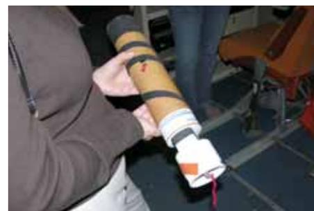
View of a dropsonde, the main atmospheric-profile sampling device for the hurricane-research flights. The red tag at the bottom is a covering for the temperature sensor; the red tag in the middle is a port to add external power for calibration before the drop. Each dropsonde costs about \$750; about 30 of them are typically used in a mission.
