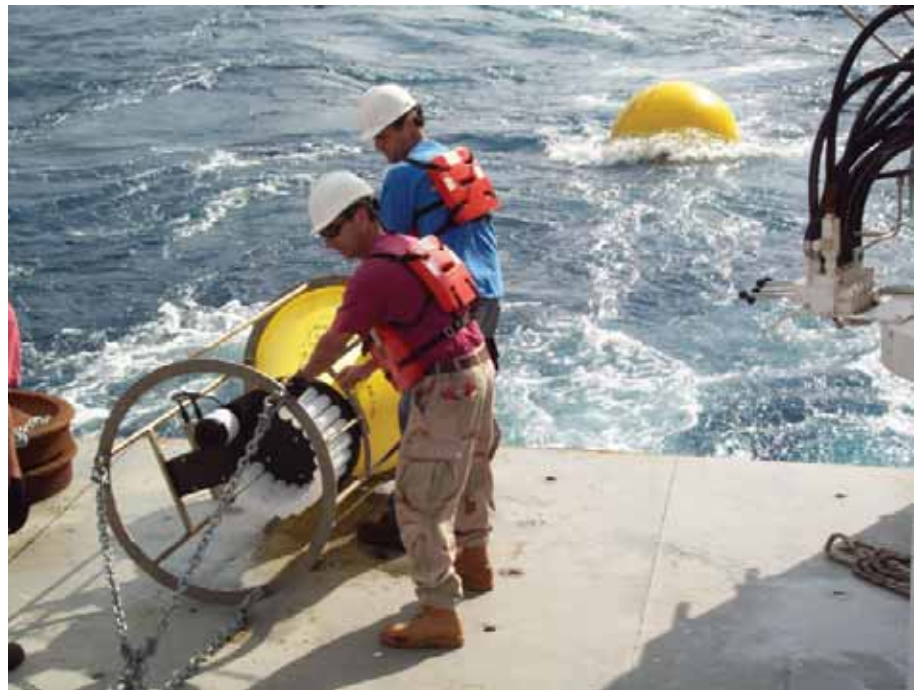
Don Hickey (USGS, left) and Eric Tappa (University of South Carolina) deploy a McLane Mark 78 sediment trap from the R/V Pelican in the Gulf of Mexico. Photograph by Wendy Kelly (USGS).
