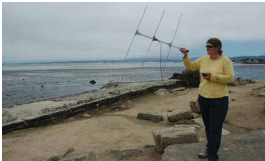
USGS wildlife biologist Alisha Kage holds out a VHF (very high frequency) radio receiver, hoping to hear the tell-tale beep that helps her locate sea otters that are part of a study to monitor and learn more about the species. Photograph by Tania Larson , USGS.
