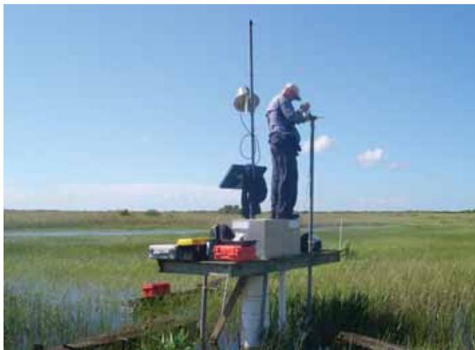
*Hydrologic technician **Gordon Anderson**, a member of **Smith's** team, repairs a rain gage at the USGS hydrologic-sampling station (a.k.a. “hydro platform”) near the Harney River. Note planks laid over sawgrass marsh to facilitate access to platform.*
