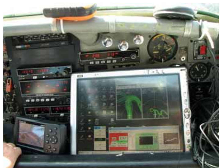
Dashboard view of incoming data from the Experimental Advanced Airborne Research Lidar (EAARL)’s unique data-collection system, which can acquire detailed elevation information from both land and shallow seafloor.
