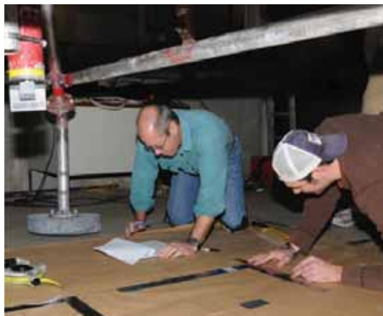
Chris Sherwood (left) and UNH master's degree student Gary Margelowsky measure instrument positions and record tripod feature locations. The fan-beam sonar is visible in the top left of the image.
