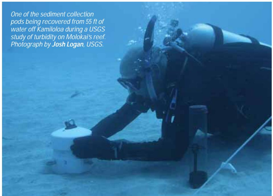
One of the sediment collection pods being recovered from 55 ft of water off Kamiloloa during a USGS study of turbidity on Molokai's reef. Photograph by **Josh Logan**, USGS.
