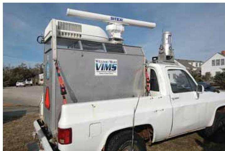
*CLARIS (Coastal Lidar and Radar Imaging System) uses lidar (light detection and ranging) to measure coastal topography and X-band radar to estimate offshore bathymetry (water depths).*
