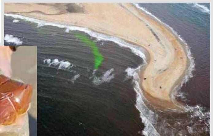
*Dissolvable bags containing uranine dye were launched into the surf zone. Aerial photographs revealed the path of the tracer (bright green) in the nearshore.*
