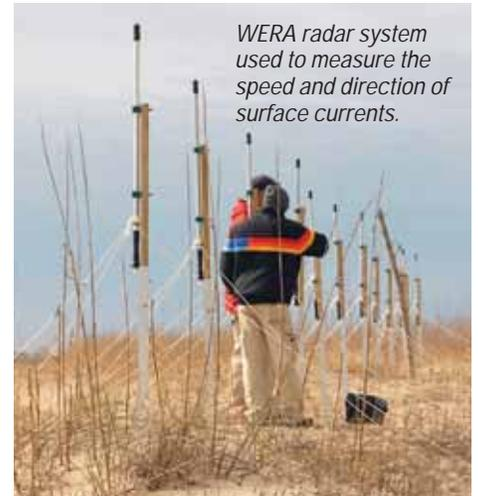
*WERA radar system used to measure the speed and direction of surface currents.*
