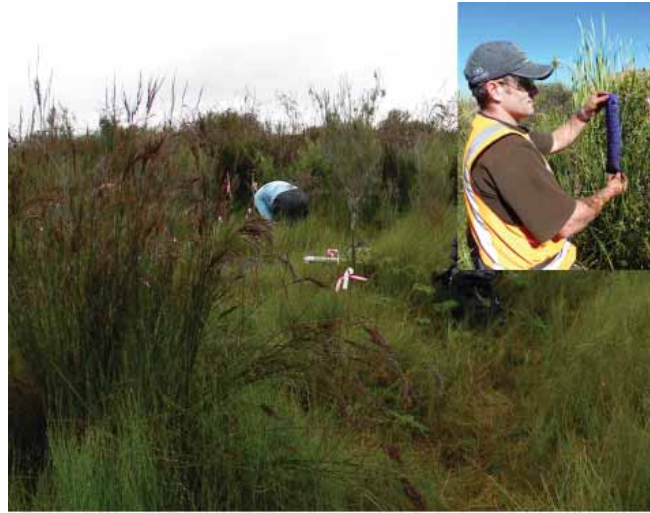
New Zealand and USGS scientists are studying how nutrient inputs are affecting freshwater bogs, especially peat formation. Scott Bartlam (inset) is holding a root ingrowth bag, which will be used to measure belowground (root) production.
