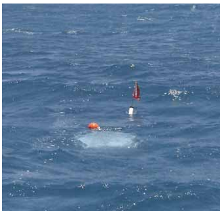
A satellite-tracked GPS drifter off Diamond Head, O‘ahu, just before recovery. The electronics are housed in the orange sphere, the large white diamond is the drogue that is calibrated to make the entire package drift at the same speed as the currents. Photograph by Josh Logan (USGS).
