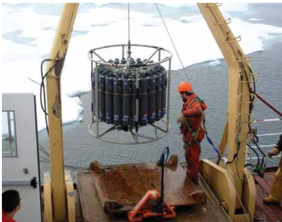
Scientists use a rosette off the deck of the Healy to take Arctic Ocean water samples.
