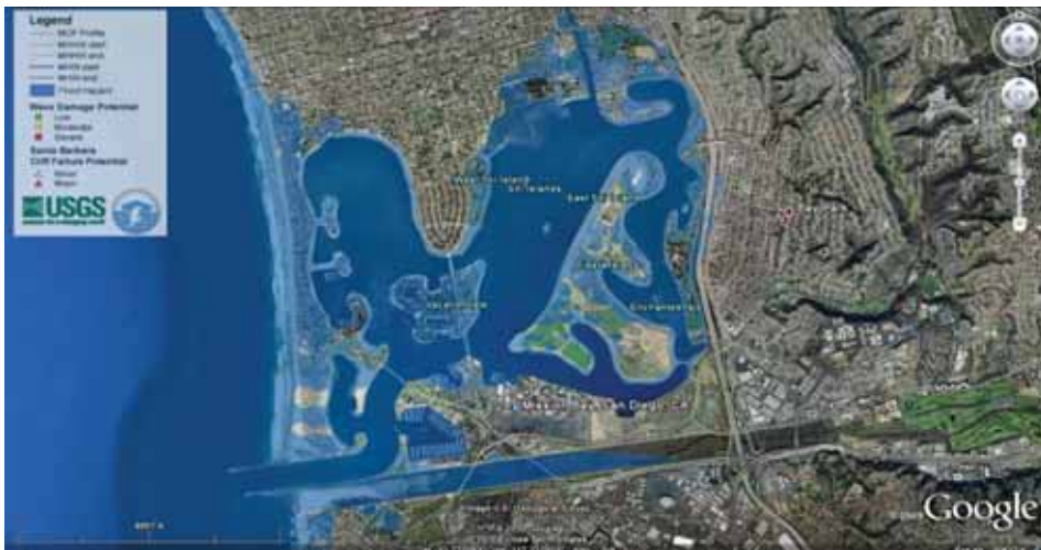
Estimated coastal inundation (blue shading) at Mission Bay in San Diego, California, using the Coastal Storm Modeling System (CoSMoS) developed for ARkStorm. (From USGS Open-File Report 2010-1312, http://pubs.usgs.gov/of/2010/1312/ )
