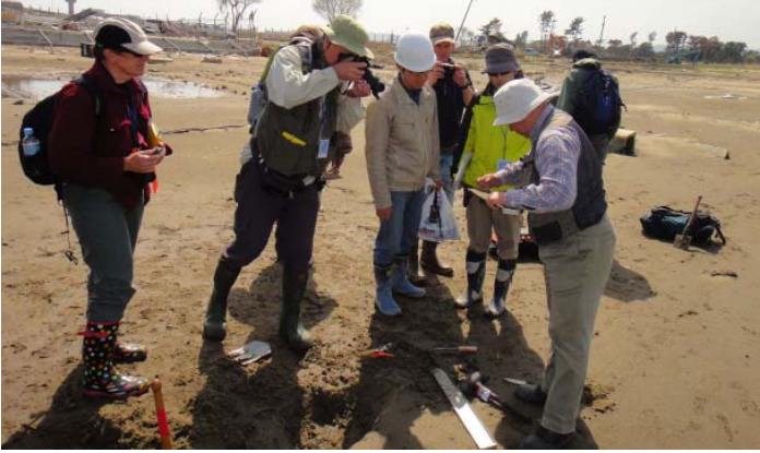
Yuichi Nishimura shows other members of the international tsunami survey team a sediment core taken by the geoslicer, a tool used to search for ancient tsunami deposits.
