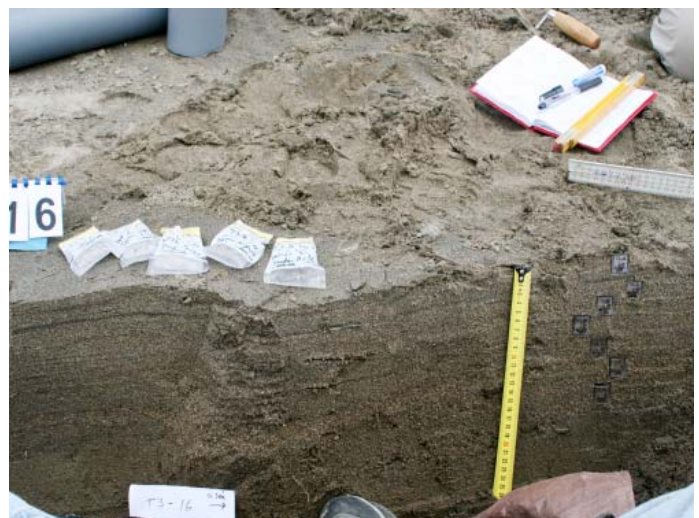
Wall of excavated trench showing the sedimentary structures of a tsunami deposit (mostly horizontal sand layers) and locations (rectangular markers on right) where sediment samples were collected for laboratory analyses.
